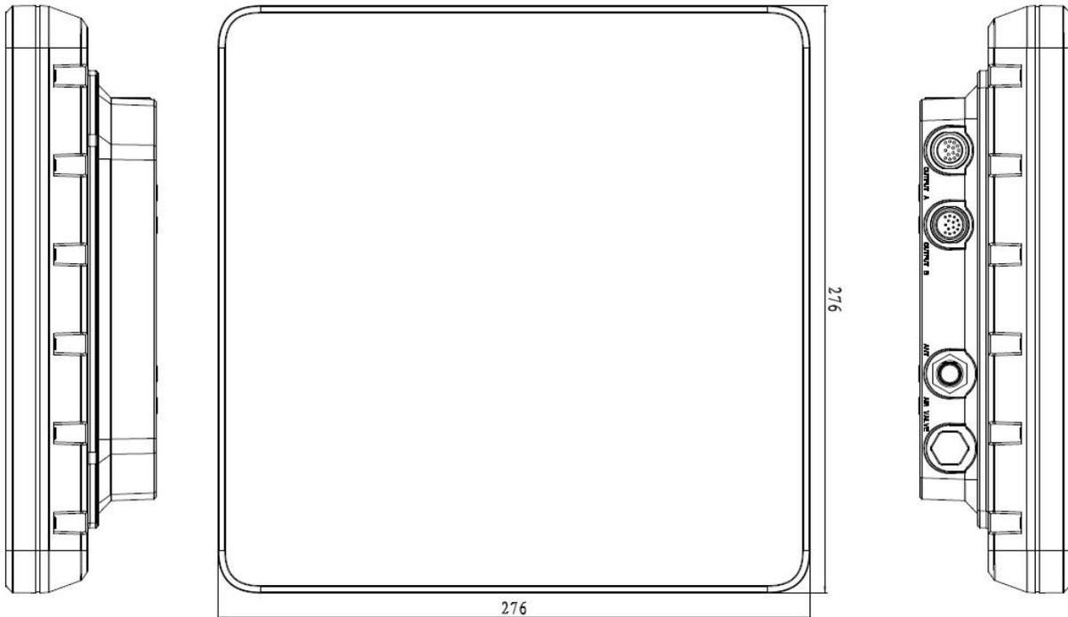
Figure 2-1 Structure diagram of Sharp 100 reader
