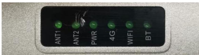
Figure 2-2 Schematic diagram of reader LED indicator panel
