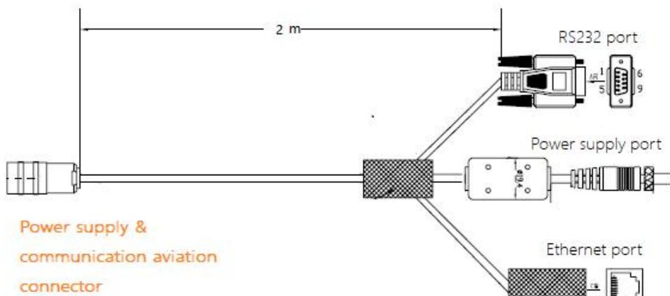
Figure 2-3 Power and communication interface cable decomposition
