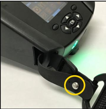
2. Insert the hole on the end of the strap over the metal post (circled) to secure.
