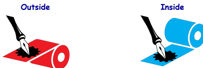
Figure 7 • Ribbon Coated on Outside or Inside
